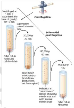
At lower speeds, the pellet consists of larger components, and higher speeds result in a pellet with smaller components.
