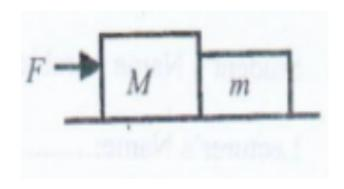
**40.**In the figure mass m=2 kg and the coefficients of static and kinetic friction are Us=0.4, uk=0.2 respectively. The acceleration in  $(m/s^2)$  of mass m is:
