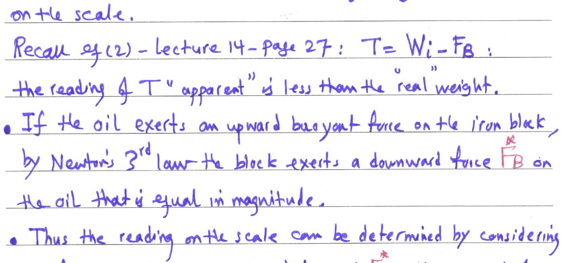
the forces acting on the oil, Wo and FB, the weight of the beaker, and the upward force from the scale o which sum to zero because the whole system is in equilibrium.  $F_{B} = P_{0}V_{i}g = P_{0}[m_{i}]g$ : Frale = Wo + Wb + FB.  $= \begin{pmatrix} e_{0} \\ p_{i} \end{pmatrix} W_{i} \qquad 6/6$  $= 39 + (l_{e_i})W_i$
