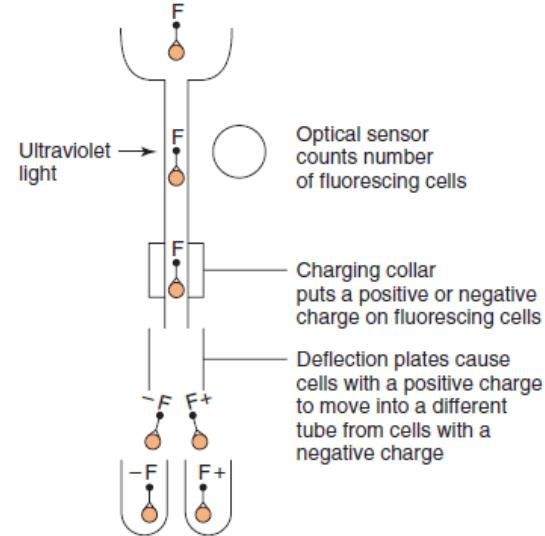
**FIGURE 64-10** Flow cytometry. At the top of the figure, a cell has interacted with monoclonal antibody labeled with a fluorescent dye. As the cell passes down the tube, ultraviolet light causes the dye to fluoresce and a sensor counts the cell. Farther down the tube, an electrical charge can be put on the cell, which allows it to be deflected into a test tube and subjected to additional analysis.
