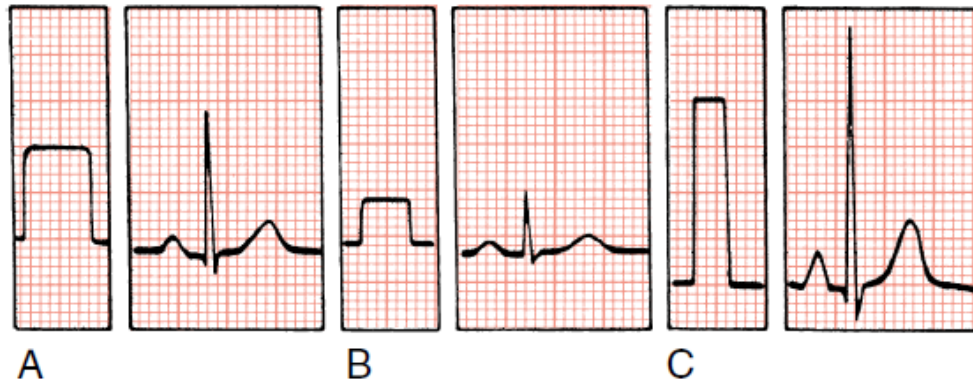
Figure 2-5. Before taking an ECG, the operator must check to see that the machine is properly calibrated, so that the 1-mV standardization mark is 10 mm tall. A , Electrocardiograph set at normal standardization. B , One-half standardization. C , Two times normal standardization.
